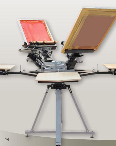
Printing begins when the garment is placed on a palette. The screen is lowered into place and the ink is squeezed through the screen onto the garment's surface. The palette is then moved to the next screen that will apply the next color, and so on, until the design is complete.
